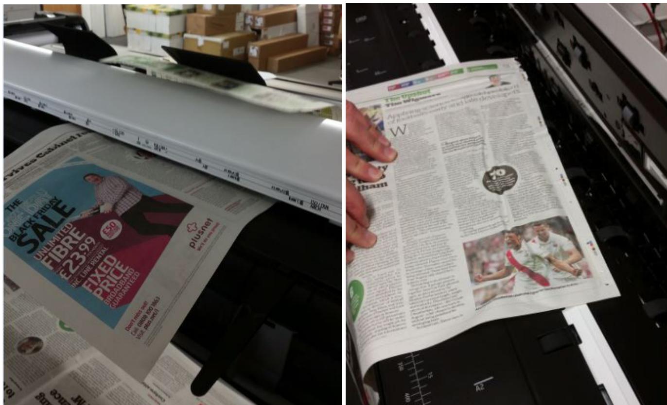
However, the Canon TM-300 MFP L36ei (shown left) successfully scanned the newspaper in portrait orientation, but the HP T830 MFP (right) could not.
