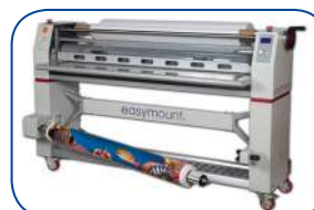
Front mandrel swings-out for easier loading of vinyl
